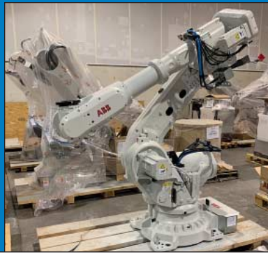
(7) ABB IRB 6700-150/3.20 Six-Axis Pedestal Type Robots
