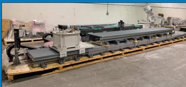
(6) ABB IRB 6700-150/3.20 Six-Axis Track Mounted Robots
